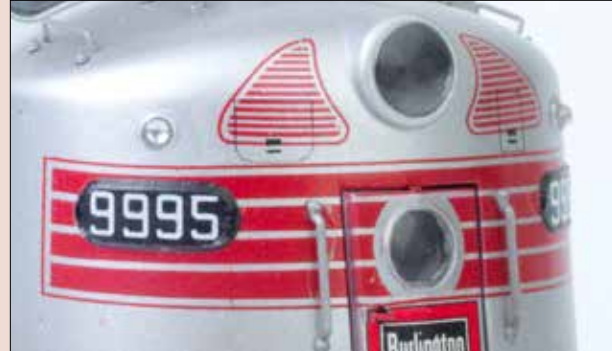
The finished decals look like the outline of the nose m.u. hatches. The model also received new number boards.
