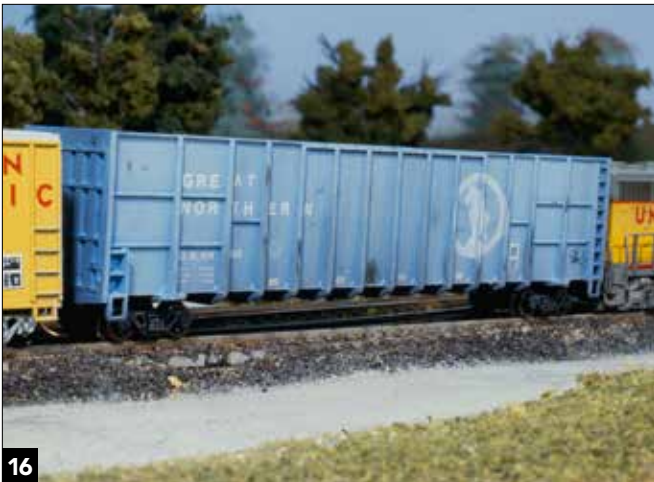
The faded paint effect on this N scale Great Northern wood chip car was created with a thinned white overspray. The car also received some rust-color drybrushing.
