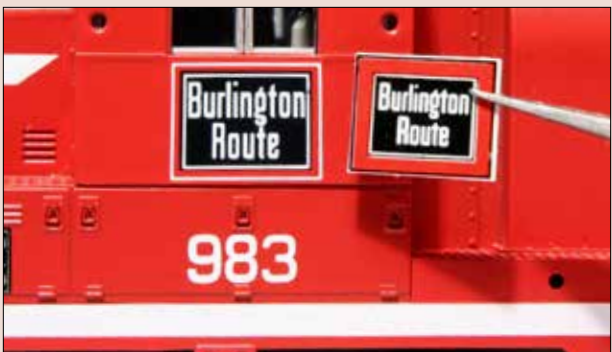
The Microscale decal at right was far more accurate than the factory-painted herald on the Kato shell.
