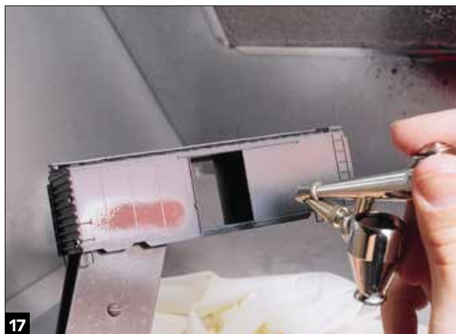
Each airbrush stroke should slightly overlap the previous one. The paint should stay wet on the surface briefly after spraying.
