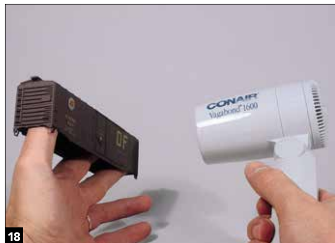
You can use a hair dryer to speed drying time with acrylics, as I am doing with the acrylic clear coat on this boxcar.
