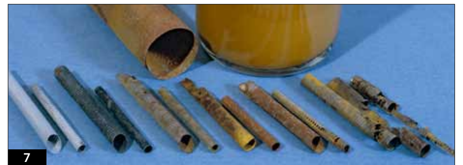
The first two pipes are "new." The others show the various degrees of corrosion achievable with etchant and the rust solution. The pipes with marvelous holes and loops of single ribs are slated for trash heaps surrounding replaced pipes along the right-of-way.
