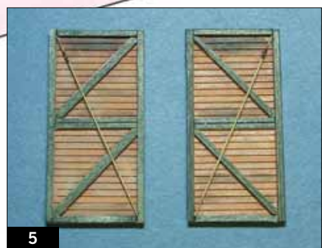
5 My friend Dave Montgomery built the flood-control doors from stripwood, scribed wood panels, and brass wire.
