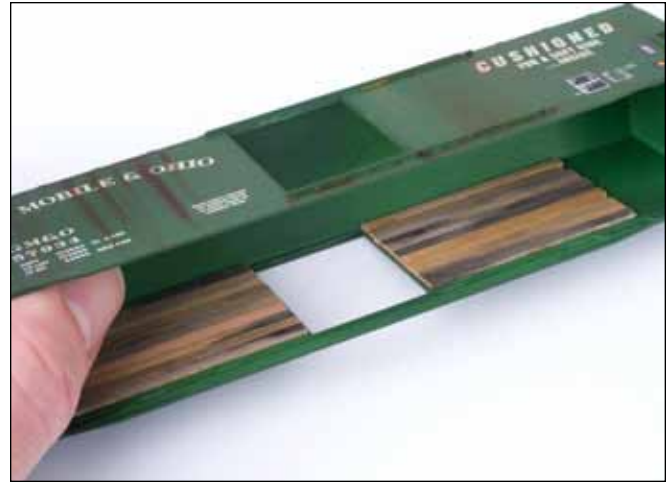
The interior walls don't have to extend to the end—just make sure they cover the normal viewing range.
