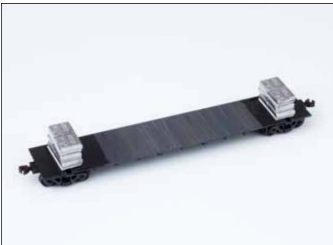
Paint and weather the floor where it will be visible. The A-Line peel-and-stick weights will be out of sight on each end.
