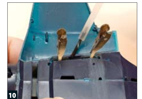
10 The upper wing half is held in place while liquid plastic cement is applied. The slow setting time of the cement allows any necessary adjustments.
