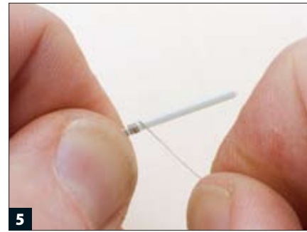
5 Tightly wrap fine wire around a piece of Evergreen square strip styrene.
