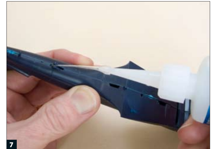
6 Using the stretched nylon nozzle, super glue is applied to the interior surfaces using any opening available.
