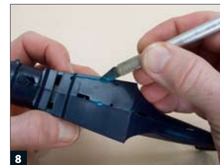
8 With holes drilled to mark the front and rear limits of the cut to be made, a saw blade essentially connects the dots.
