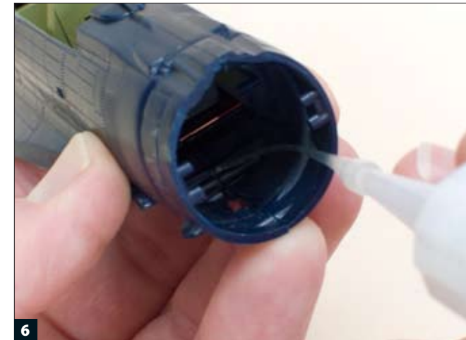
6 Using the stretched nylon nozzle, super glue is applied to the interior surfaces using any opening available.
