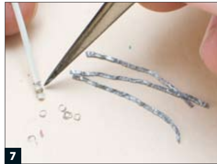
7 The cut loosens the squares enough to be coaxed off the strip stock with fine tweezers. These same tweezers will be used to force the cut ends back to touching each other, reforming visually intact squares.
