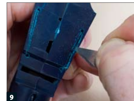
9 The resulting slot is carved open with a hobby knife with a No. 11 blade.
