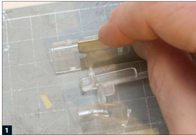
1 With a cushioned cutting mat underneath, a single-edge razor blade is applied to the sprue joint like a guillotine, making a perfectly clean separation of the canopy.
