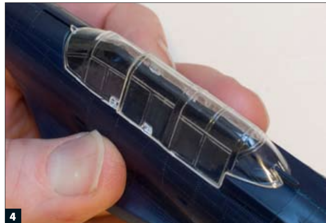
4 Test-fitting the canopy early in the building process alerts you to fit problems that you may encounter at the end of the process when the actual attachment of the clear parts takes place.
