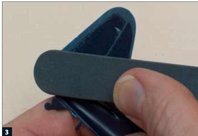
3 The same procedure is applied to all the mating surfaces of the kit, ensuring the tightest possible fit for all parts.
