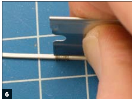
6 A razor blade works well for cutting the wire on one side of the strip. The result is a bunch of wire square "buckles."
