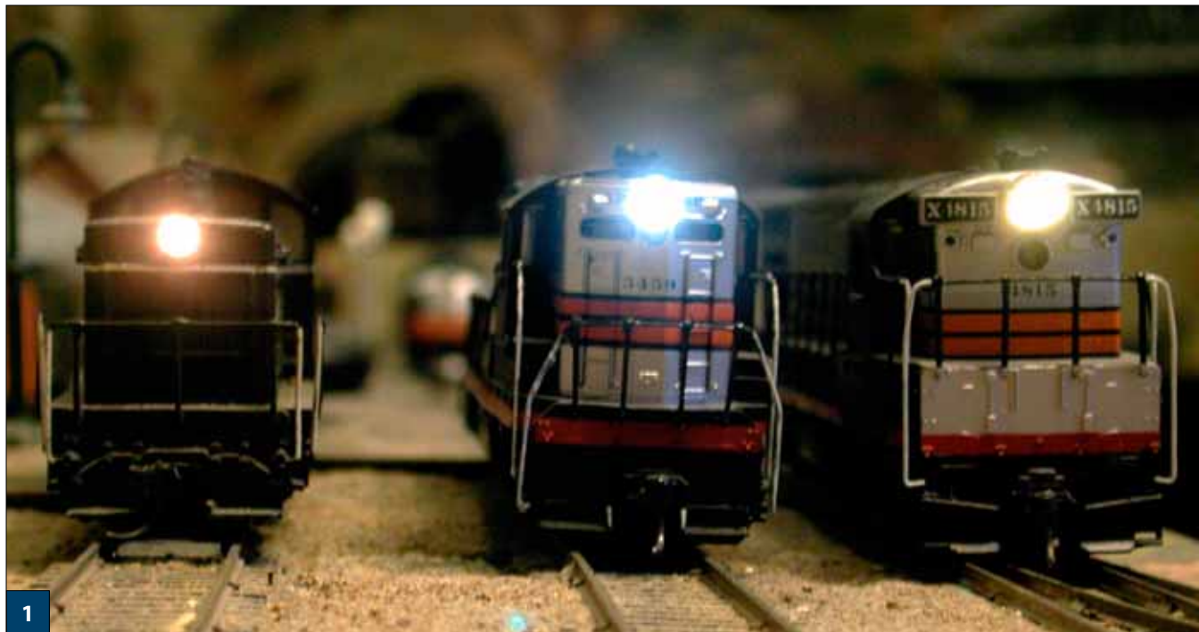
The locomotive headlight on the left is a lamp, the one in the middle is an older bluish-tint white LED, and the model at right has a Yeloglo LED that gives off a color more like an incandescent lamp.
